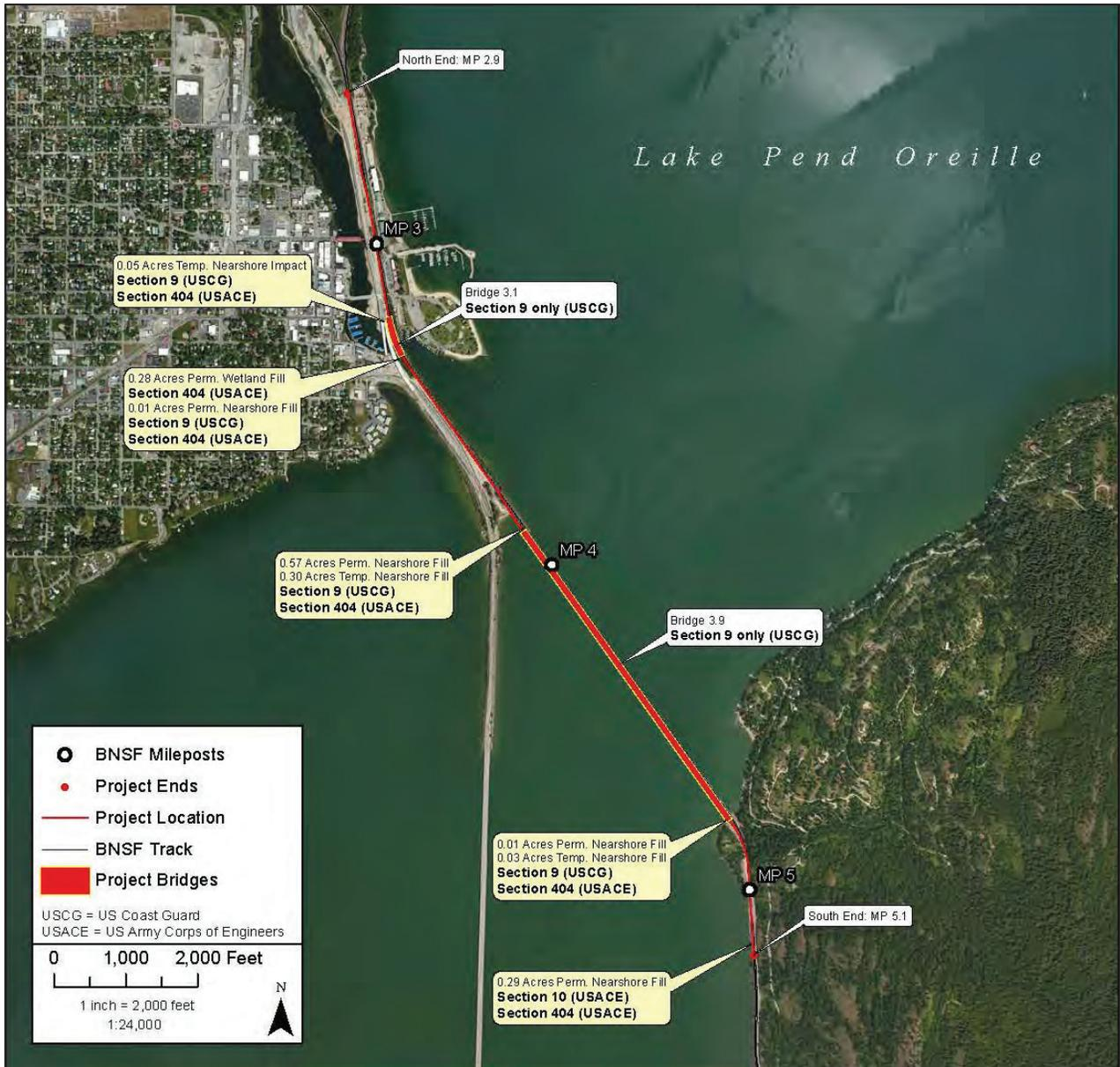
Alternative 1 is the preferred alternative that fully met the purpose and need of the project, while having the least environmental impacts. Table 2 below summarizes the Design options that were reviewed at each of these locations. The area reduction of nearshore fill through design adjustments resulted in a total reduction of 1.97 acres of permanent fill and 0.17 acres of temporary fill.
